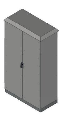
Thanks to the IP 55 protection level and electrostatic paint coating, the cabinet provides protection against external conditions, adversely affecting the mounted devices. Side walls, doors and roof are made of 2 mm aluminum
