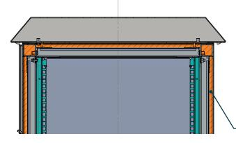
The construction of the side walls and profiles enables the use of additional insulation in order to reduce the Lambda heat transfer coefficient
