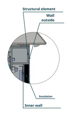
Double structure with doors, roof and side walls made of 2 mm aluminum
