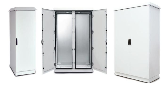
**Application:**The STREETBOX series are outdoor distribution cabinets made of powder-coated aluminum. Double-layer walls, a high degree of protection and electrostatic painting provide optimal protection for the devices installed inside.
